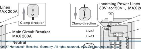
The installation of your Aeotec Home Energy Meter has two major parts: the installation of the meter into your Z-Wave network, and the installation of it into your AC mains electricity box. The electrical installation of your meter into your circuit box should only be done a licensed electrician with knowledge and understanding of electrical systems and electrical safety. You can perform the second half of the installation process, linking the meter with your Z-Wave network, yourself.
