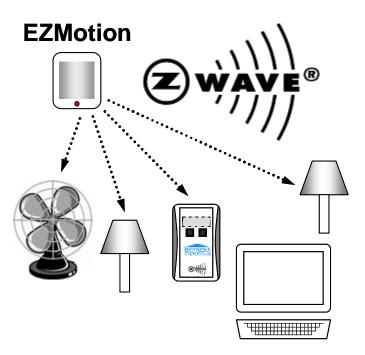
In addition to the motion sensor, EZMotion also senses the amount of light in the room as well as the current temperature. The light sensor of EZMotion can be programmed to leave the lights off if there is already sufficient natural light in the room. The thermometer feature of EZMotion can be used to adjust the heating and cooling system to keep the room comfortable.
