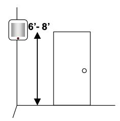
person sitting in front of a computer or reading in a comfortable chair will not be moving enough for EZMotion to detect unless it is placed close to the person. The sensitivity of EZMotion can be set to high or the time delay when lights are turned off can be made fairly large (1 hour or more) to compensate for situations where people are sitting still. The best location is usually in the corner of the room adjacent to the entry door.
