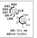
With the top rotary switch in the setting LRN up to 35 wireless pushbuttons can be assigned therefrom one ore more central pushbuttons. The required function of this impulse group switch can then be selected:
