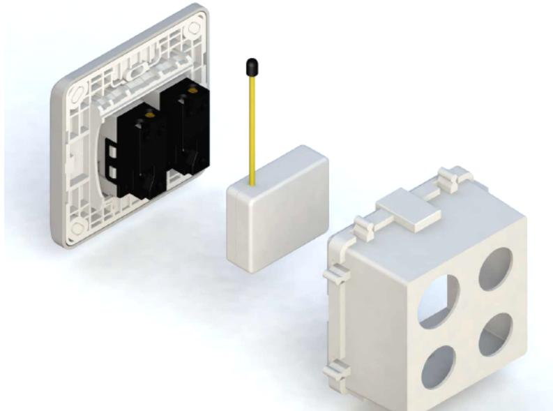
Put the in wall switch into a wall box and connect the pins as shown in the figure.
