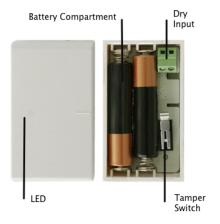
Attention: The electronic circuit of the MTemp can be damaged in the case of wrong insertion of batteries.
