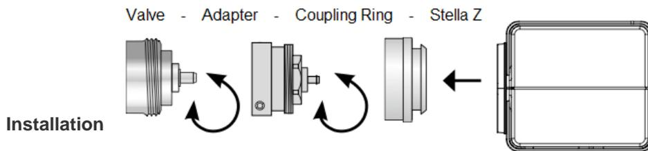
The installation of the valve control is easy with any dirt or loss of water since the heating pipe system will not be interrupted.
