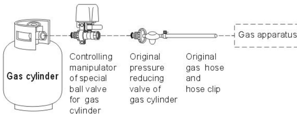
4. When the gas alarm failure, pull down the clutch(knurling round nut of the manipulator), and then manually turning the handle to 90 degree to open the valve until the handle rotates to the dead point. Then, remove your fingers from the round nut and gently move the handle to make the clutch back to its original position.
