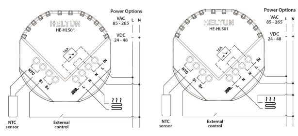
Figure 4: Connection diagram 1
