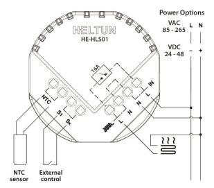
Figure 3: Connection diagram 2
