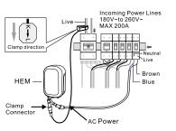
In 230 volt countries with a 3 phases and 3 wires installation:
