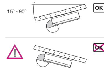
**Installing the ARGUS on corners and fixed pipes**
