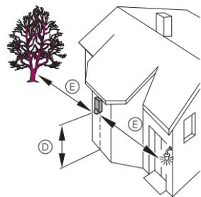
**Mounting height (D): 2-3 m.** For optimum monitoring, we recommend a height of 2.5 m on a solid and even base.
