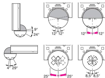
2 From its edge step into the area of detection to see whether the ARGUS switches the load and the functional display as required.
