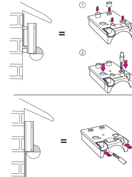
**Installing the ARGUS on the ceiling**
