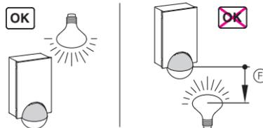
**Minimum distance (F) between luminaire and movement detector:** 5 m. If this distance cannot be achieved, you can use the segments provided to "mask" the light source from the area of detection.
