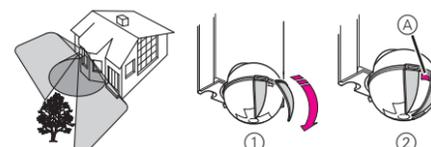
Ensure that the brightness sensor (A) is not covered, as the sensitivity to light is otherwise reduced.
