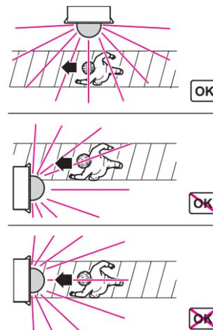
To avoid the connected load being switched on due to environmental influences, the ARGUS should be installed so that it is protected against rain and direct sunlight. A raindrop running over the lens, for example, can activate the movement detector.
