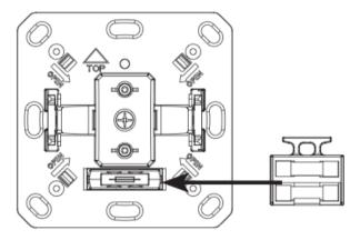
NOTE: The micro-fuse deals with a backup for the equipment that is specifically designed to this radio-controlled wireless dimmer/switch/sunblind. Please use only this fuse type. This micro-fuse should protect this radio-controlled wireless dimmer/switch/sunblind from overload and short circuits. When using another fuse component there is a danger that the device can be destroyed. A spare fuse is provided in the fuse holder.
