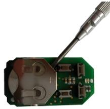
For battery change the device needs to be opened by removing the three little screws on the back side of the device. Use a screw driver or any other usable device to gently push out the battery as shown on the picture. During reassembly watch the position of the white rubber and the make sure the silver buttons fit exactly into the nipples of the rubber.
