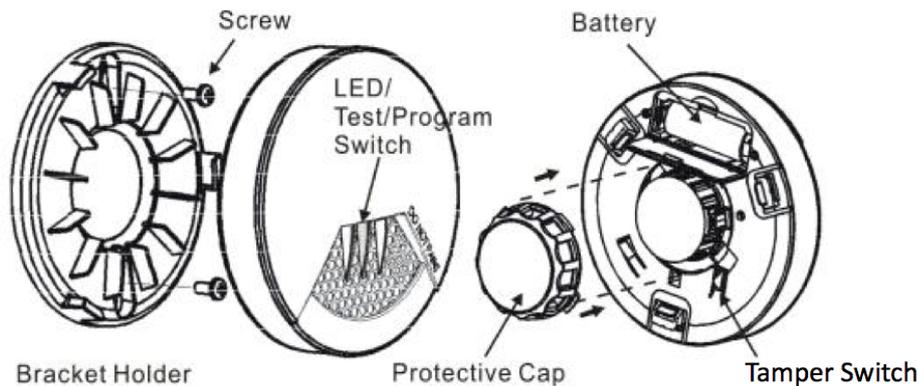
Remove the bracket from the detector by rotating it counter-clockwise.
